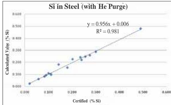
Figure 2: Silicon in steel using the Niton XL3t GOLDD+ analyzer with He purge.
