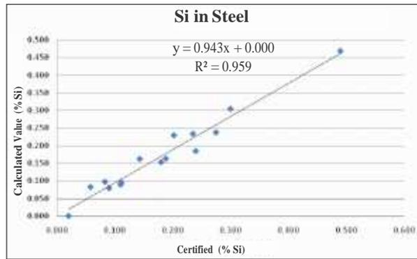
Figure 1: Silicon in steel using the Niton XL3t GOLDD+ analyzer.
